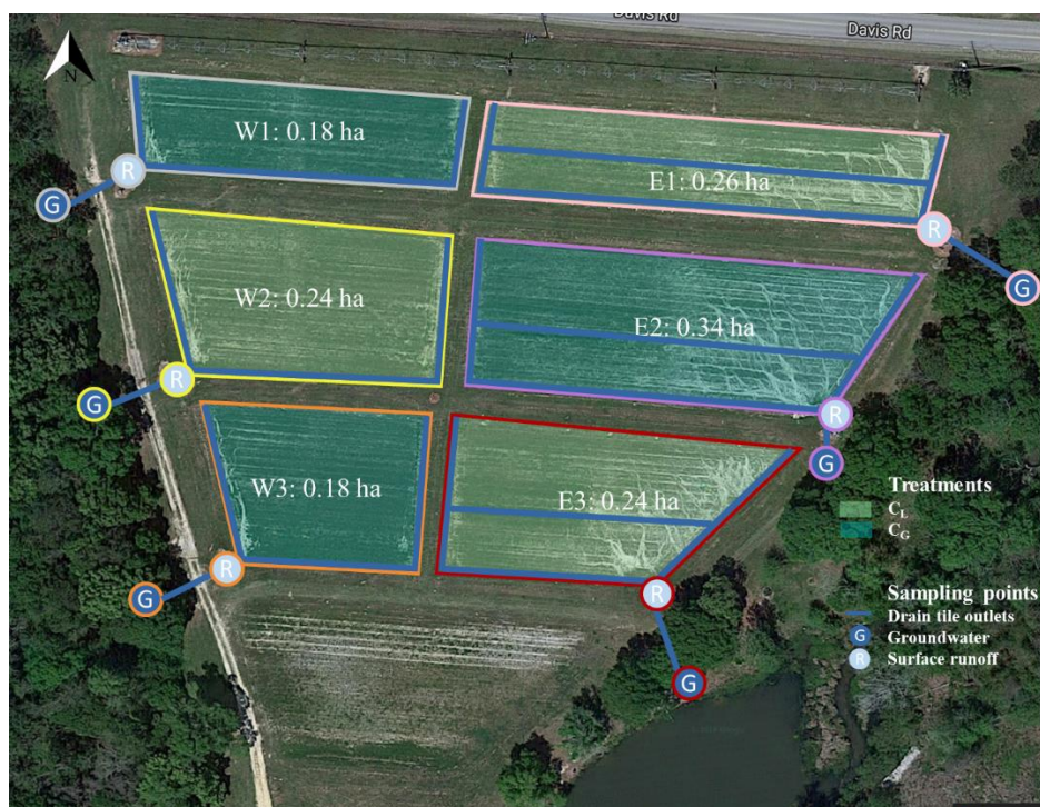
Figure 2.1 C E (light green) and C G (dark green) fertilization treatments, location of the drain tiles outlets with blue lines. Sampling points for groundwater and runoff. Blocks of NESPAL field.
