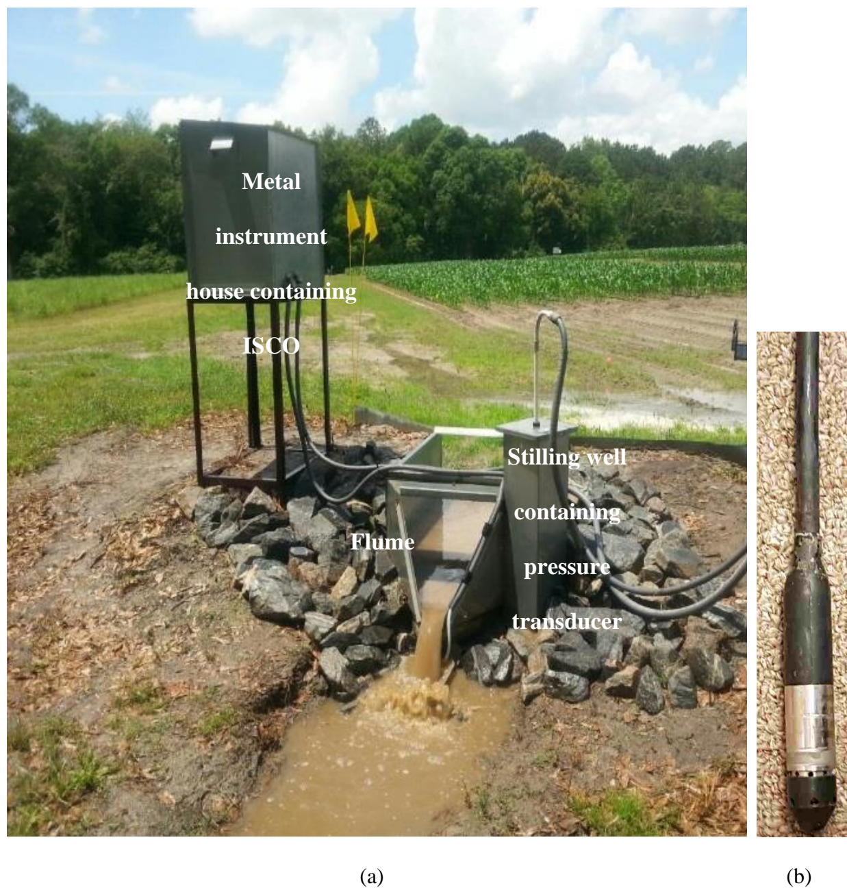
Figure 2.5 (a) Equipment used for flow proportional runoff sampling and (b) pressure transducer.
