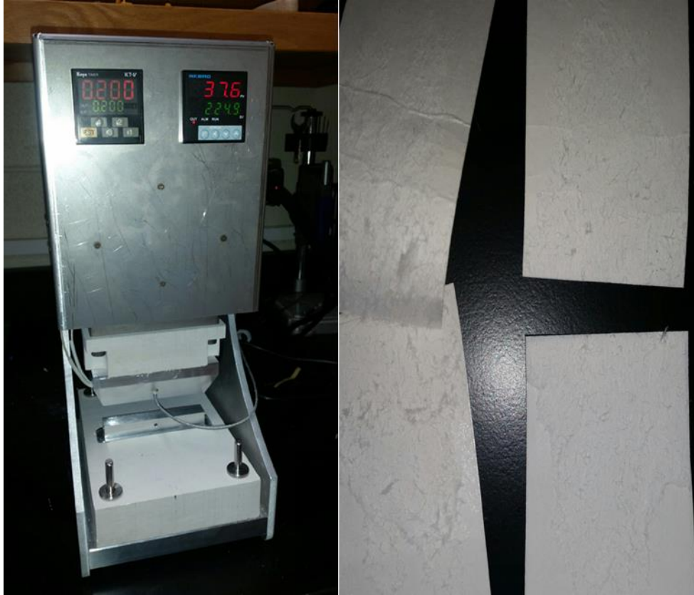
Figure 2-13: Picture of Heat Sealer Designed according to ASTM F2029 for testing heat sealing of paper coatings and example of heat seal sample demonstrating full fiber tear.
