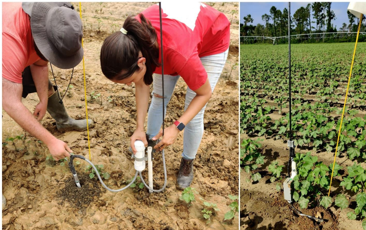
Figure 3.2. Field installation of UGA Soil Sensor Array (SSA) node.
