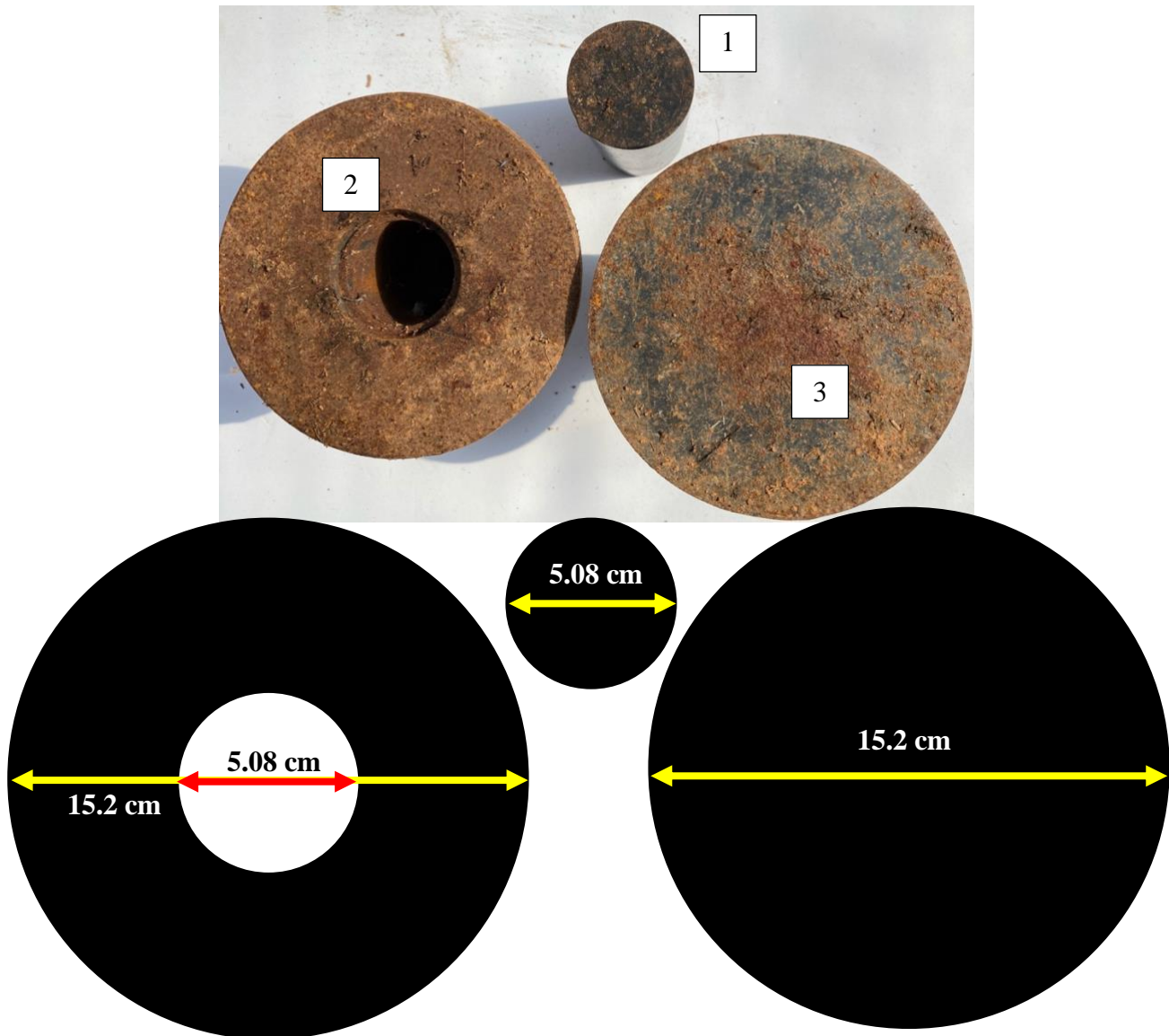
Figure 3.1. Compaction foot used in this study that attached to the pneumatic press and compacted the crown only (1; C), soil only (2; S), or crown and soil (3; CS). The C foot was used to compact the crown of the plant but not the surrounding soil. The S foot was used to compact the soil surrounding the plant, but not the crown of the plant. The CS foot was used to compact both the crown of the plant and the surrounding soil. The device was set to uniformly apply 207 kPa of downforce.
