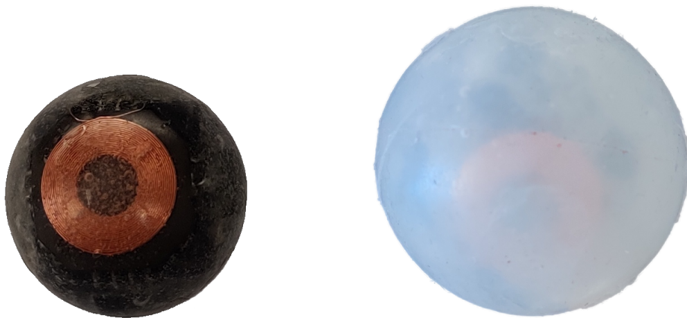
Figure 7.5: Inner (left) and outer sphere (right) of the BIRD Next sensor.
