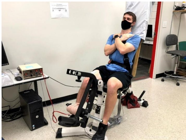
Appendix K-a: Neuromuscular assessment instrumentation. Participants were secured at the lower leg, waist, and shoulders to the custom-fabricated dynamometer. The dynamometer output (torque) was read by the custom TestPoint software, and the electrical stimulator pictured was computer-operated by the software.
