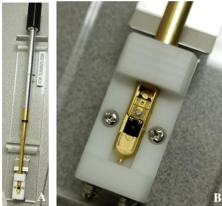
Figure 3: A) Sample holder for the Hitachi SU9000EA. B) Close up of the sample holder where the chip is housed.
