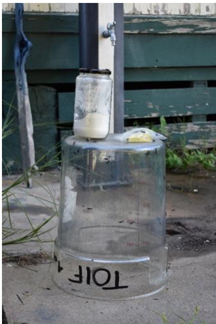
Figure AA.4. Calcium hydroxide to increase alkalinity in the vat and litmus papers to test pH.
