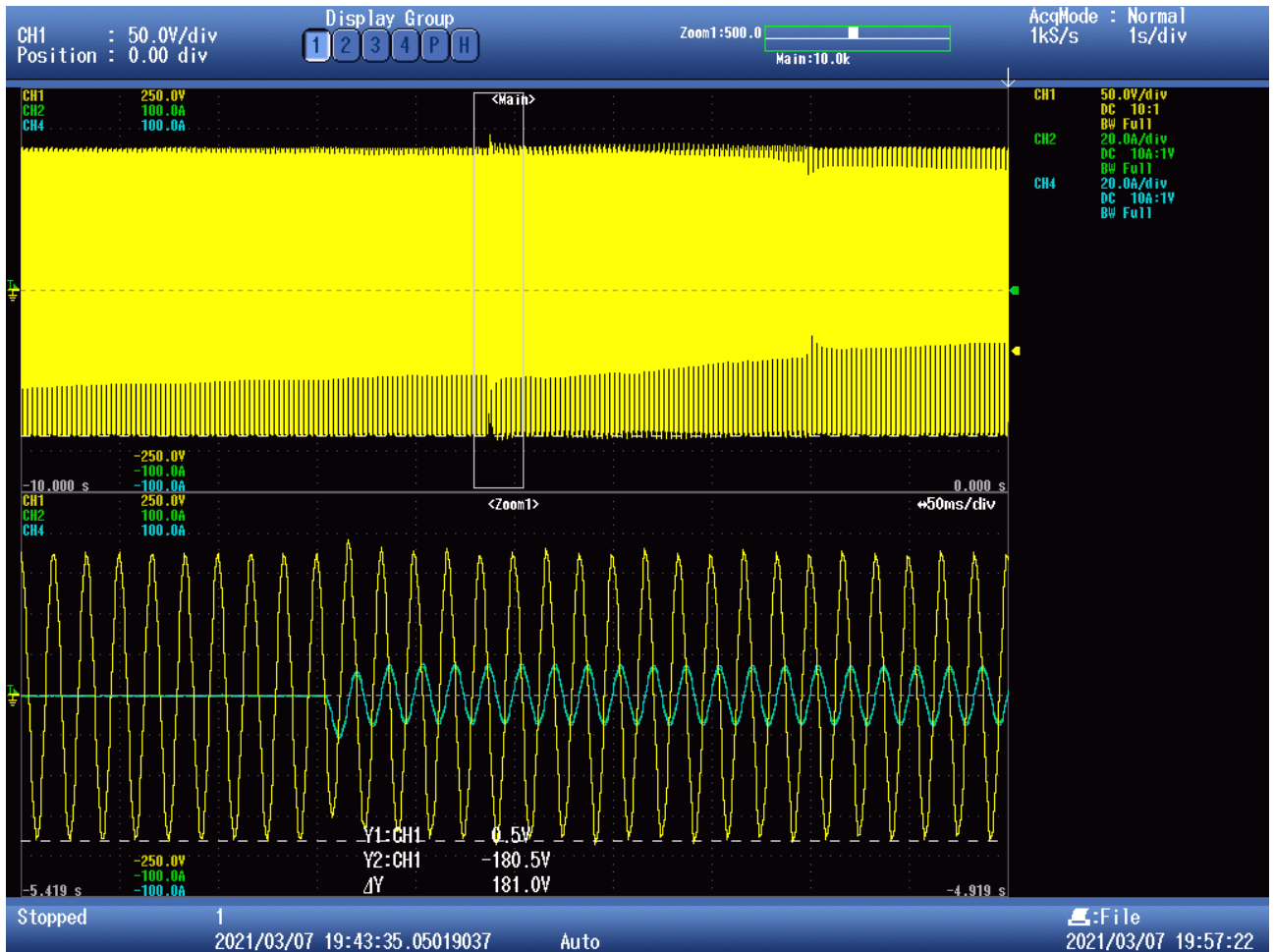
Figure 2.10: Inverter-1 system response. R_{v_k} = 1 \Omega and L_{v_k} = 0 . Load transient of L_L = 14.9 \text{ mH} and R_L = 0.5 \Omega . CH1 Output voltage, u_1 . CH2, Output Current, i_1 .
