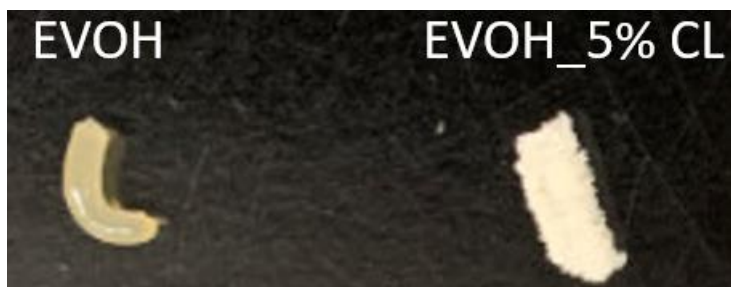
Figure 4.14. Picture of EVOH and EVOH_5% CL flushed out of extruder at 200°C.
