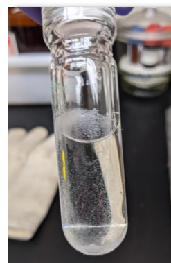
Figure 16. Picture of solid MOF material clinging to the sides of the high-pressure vessel.
