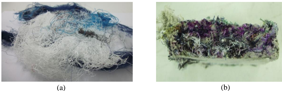
Figure 2.5. Textile waste fiber and produced board (reprinted with permission) (Adapted from [52]).
