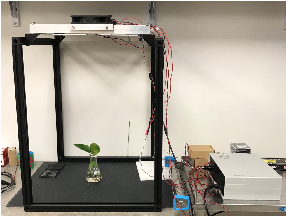
Figure 4.3: The testing setup used for all the cameras and filters. A black tarp would be used to cover the setup during testing to block out any ambient light.
