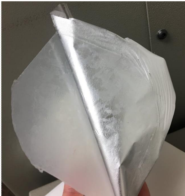
Figure 3.4 PHA (left) adhered to metallized viscose (right). Adhesive can be seen on both layers after peeling apart.
