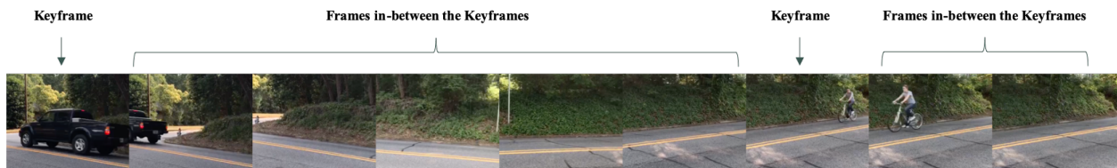
Figure 4.7: Video: Keyframes and Frames in-between the Keyframes (Keyframe is a frame used to indicate the beginning or end of a change made to a parameter).
