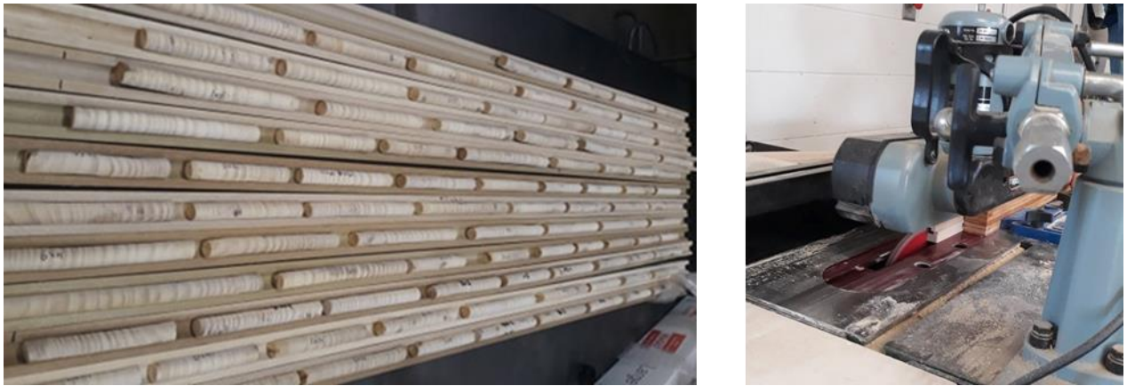
Figure 3: The samples layout in poplar core holders (left). The twin-blade table saw (right).
