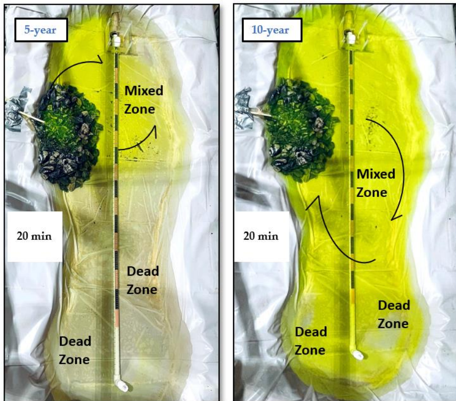
Figure 3. 7. Schematic flow pattern of the 5- and 10-year storms, right and left image respectively. Mixed and Dead zones were highlighted.
