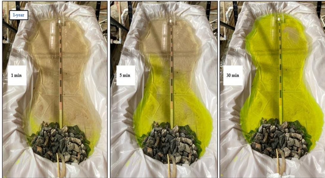
Figure 3. 8. Surface flow distribution with new inlet location for the 1-year storm tracer experiment.
