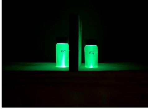
Figure 3. 4. Tracer concentration analysis with UV light.
