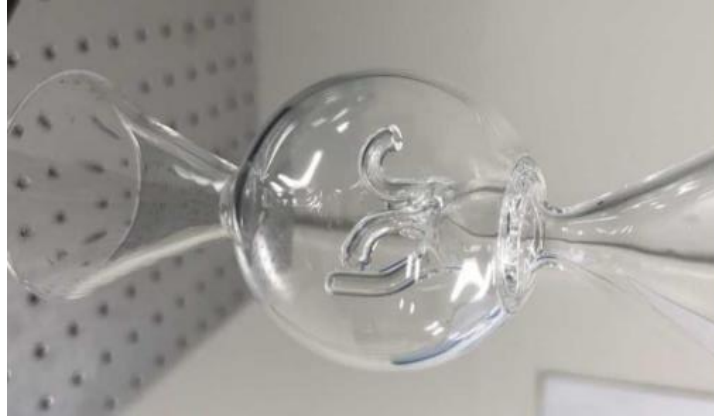
Figure 2: Jet-stirred reactor used in experimentation with four turbulent jets used for secondary mixing. Sonic probes sample from the reactor by translating from left to right in the image above.
