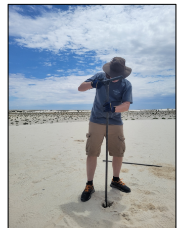
Figure 15. Dr. Bob Craddock hand-augering a borehole for well installation in WSNP.
