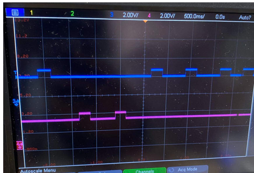
Figure 4.1. Pulses generated by the photodetector circuit recorded by the oscilloscope.
