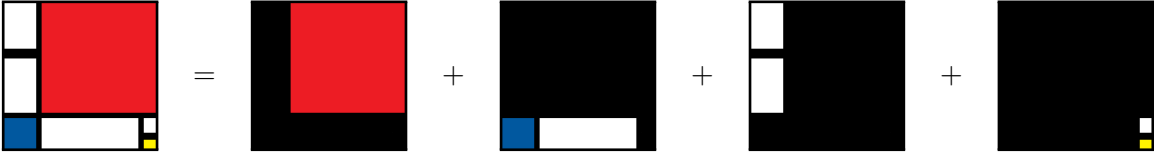
Figure 1.4: Mondrian, Piet. Composition with Red, Blue, and Yellow 1930, may be expressed as the sum of four rank one matrices. Black represents zeros.
