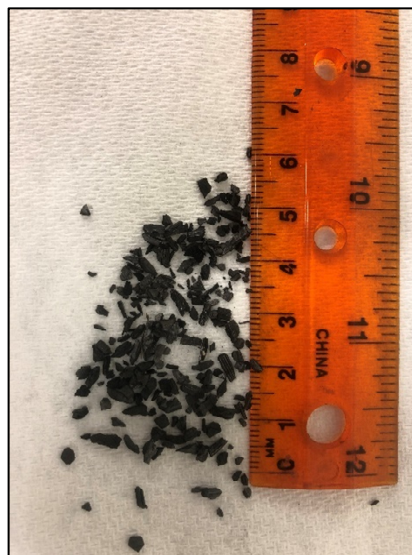
Figure 6 – Particle size of biochar ( 500\mu\text{m} < X < 2\text{mm} ) used in batch and column tests.
