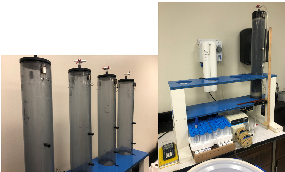
Figure 7 - Photos of plastic columns used in the column experiments.
