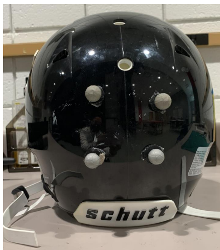
Figure 4.1b. Helmet markers placed on back of helmet.
