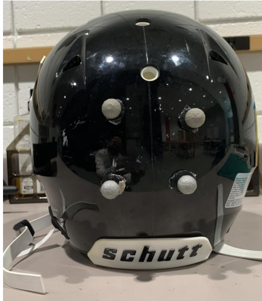
Figure 3.1b. Markers placed on back of helmet.
