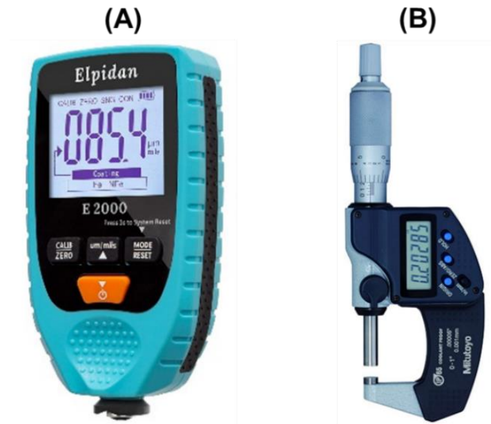
Fig. 2.4. Paint thickness gauge (A) and micrometer (B) that initially used for the measurement of coating uniformity but were abandoned due to the lack of accuracy and repeatability.
