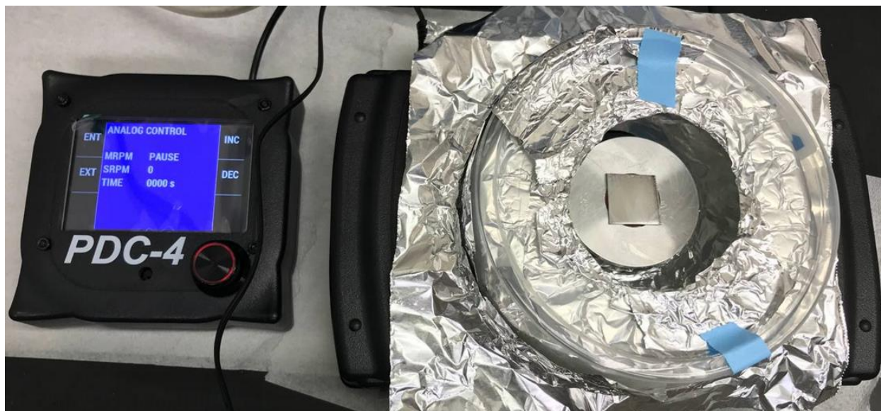
Fig. 2.7. Spin coating setup used to prepare PCL-LS coated Mg substrates.
