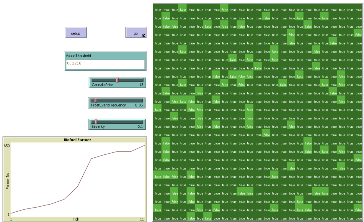
Figure 2.5: The output of a model run at carinata price $13/bu, Adoption threshold = N (0.2, 0.1216), Risk aversion = Uniform (0.5-1) after the end of the simulation period. The ‘true’ cells represent the farmers who will cultivate carinata at the end period and ‘false’ represent the farmers who will not adopt carinata.
