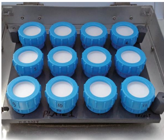
Figure 5 A custom adapter provides 12 replicate samples from each Tisch aerosol collector.
