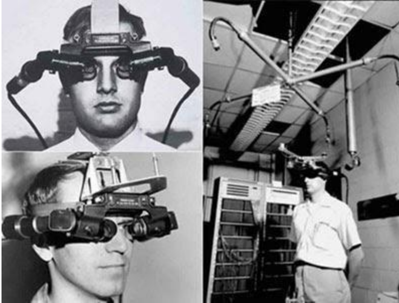
Figure 16. Sword of Damocles , 1968, -head mounted VR from Evans and Sutherland (Evans and Sutherland 2021).
