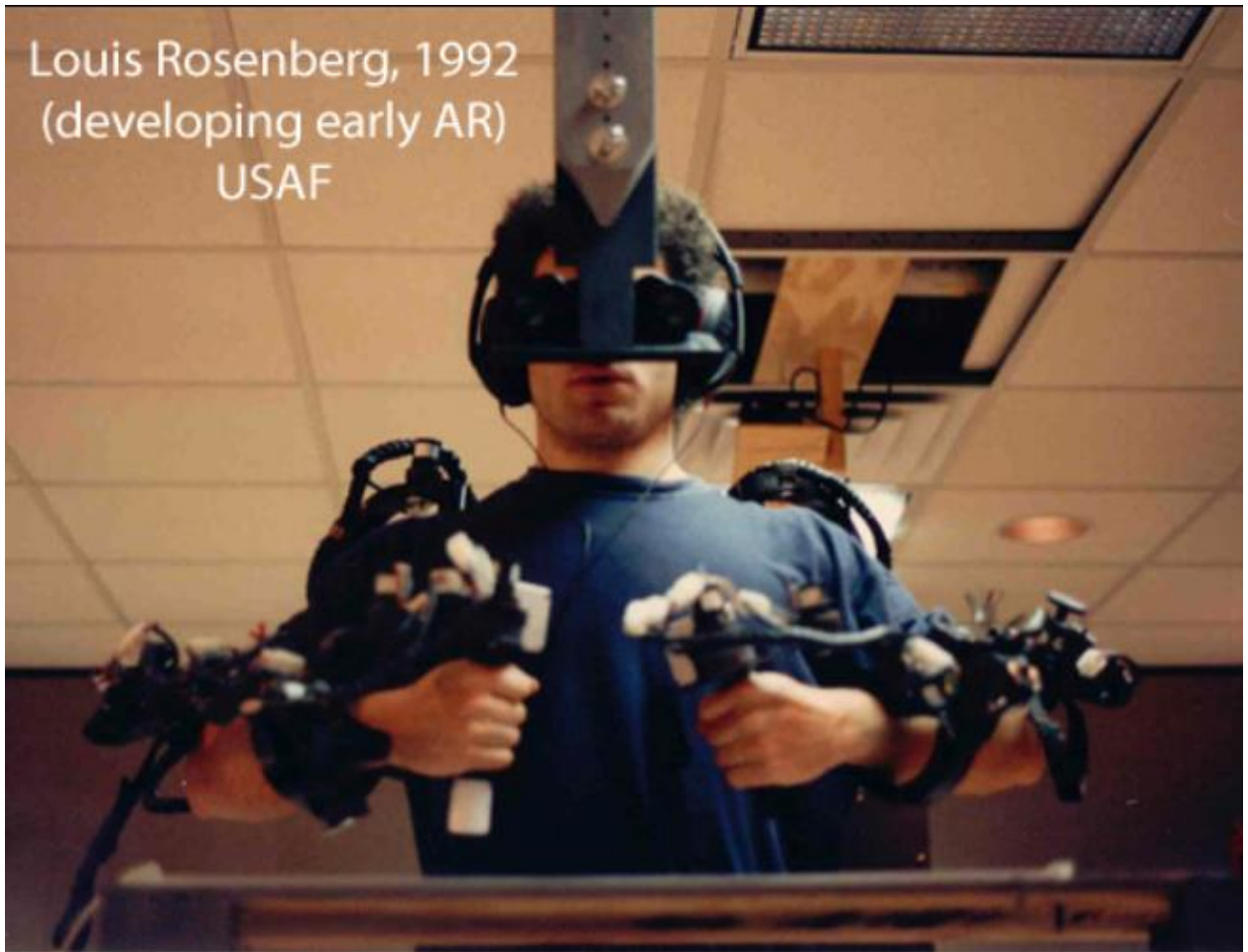
Figure 17. Louise Rosenberg used the first AR system, Virtual Fixtures, to move digital robotic arms that move relative to his real arms to research human productivity at work.
