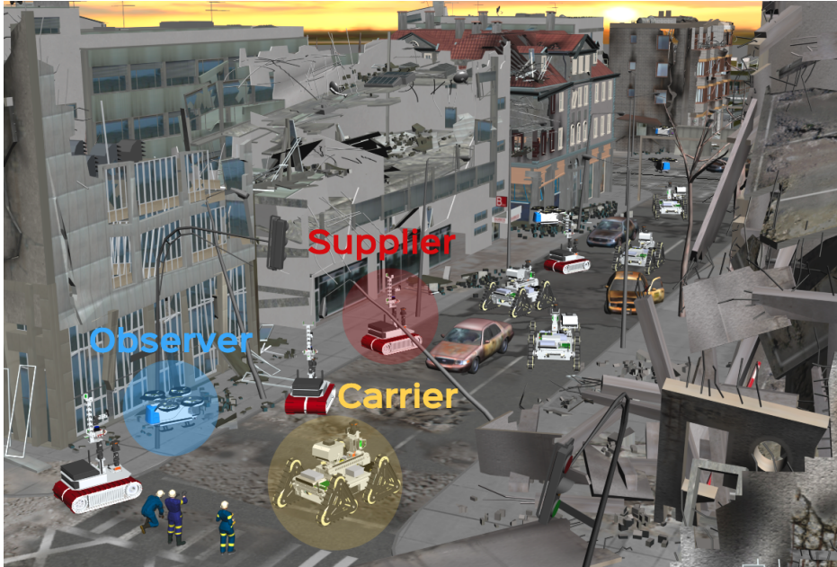
Figure 4.1: Illustration of an integrated team of robots (UGVs + UAVs) and human cooperatively working together in a post-earthquake rescue mission.
