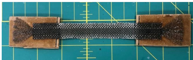
Figure 5.3. A prepared PU/WS2/UHMWPE sample for tensile test.
