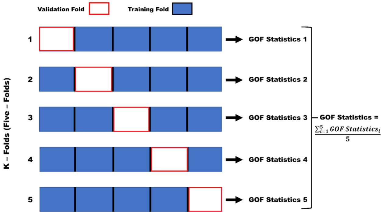
Figure 4.1. Schematic representation of five-fold cross-validation approach. Each horizontal bar is divided into five sections, out of which four are training folds and one section is the validation fold. There are altogether five horizontal bars representing five iterations or folds. Goodness-of-fit statistics (GOF) are calculated for each iteration and the final GOF statistics for a model is calculated as the average of five GOF statistics from five iterations.
