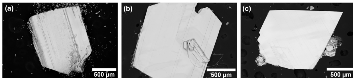
Figure 3.1 SEM imaging of single crystalline (a) \text{Hf}_{0.20}\text{Zr}_{0.80}\text{Te}_3 , (b) \text{Hf}_{0.40}\text{Zr}_{0.60}\text{Te}_3 , and (c) \text{Hf}_{0.80}\text{Zr}_{0.20}\text{Te}_3 .
