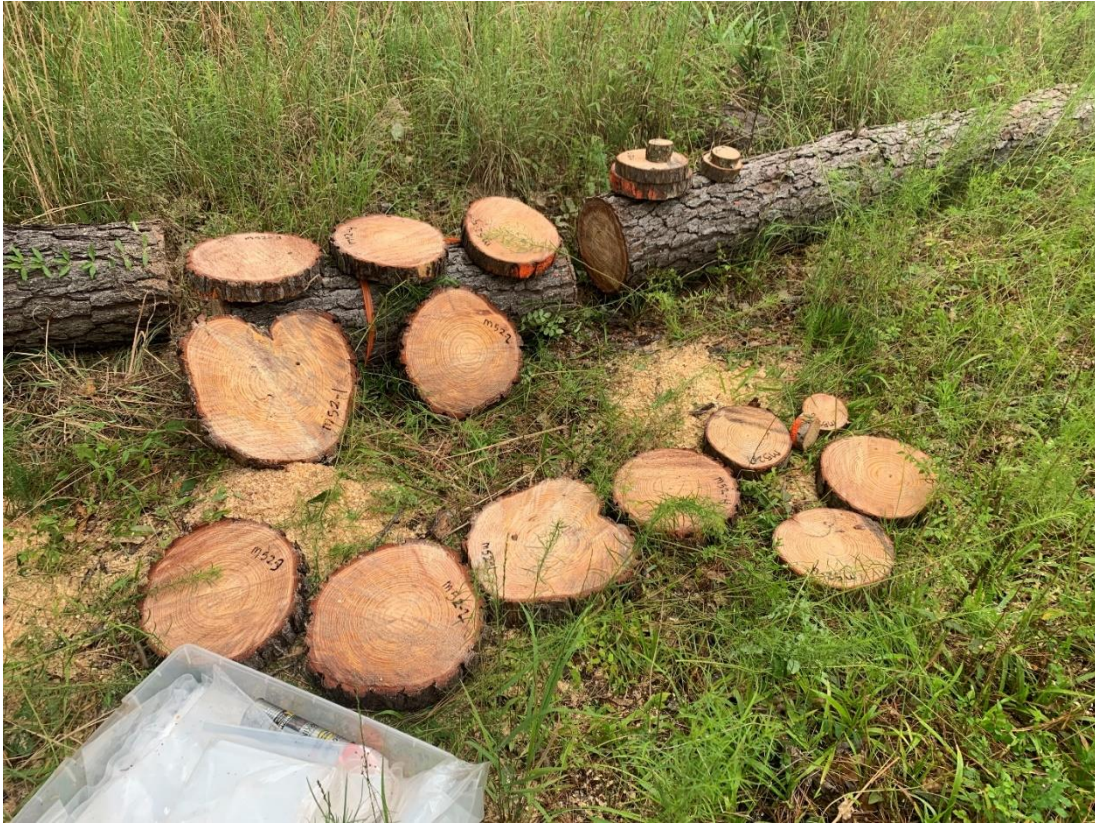
Figure 2. Example of cross-sectional disks that were collected incrementally up the tree.
