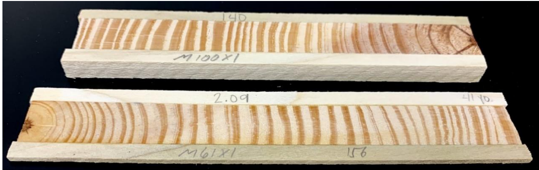
Figure 3. Radial strips used for measuring X-ray densitometry (bottom) and ultrasonic velocity (top) values.
