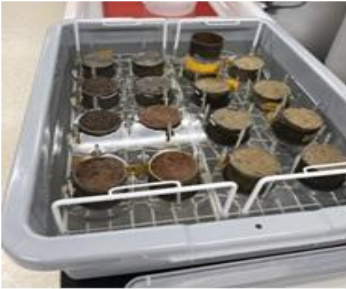
Supp. Figure 1. Saturating soil cores for field capacity tests
