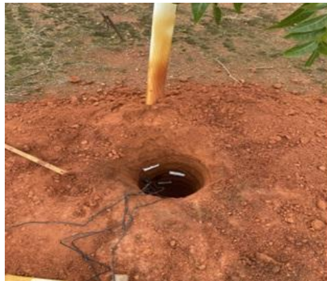
Figure 7. Volumetric Water Content Sensor Installation
