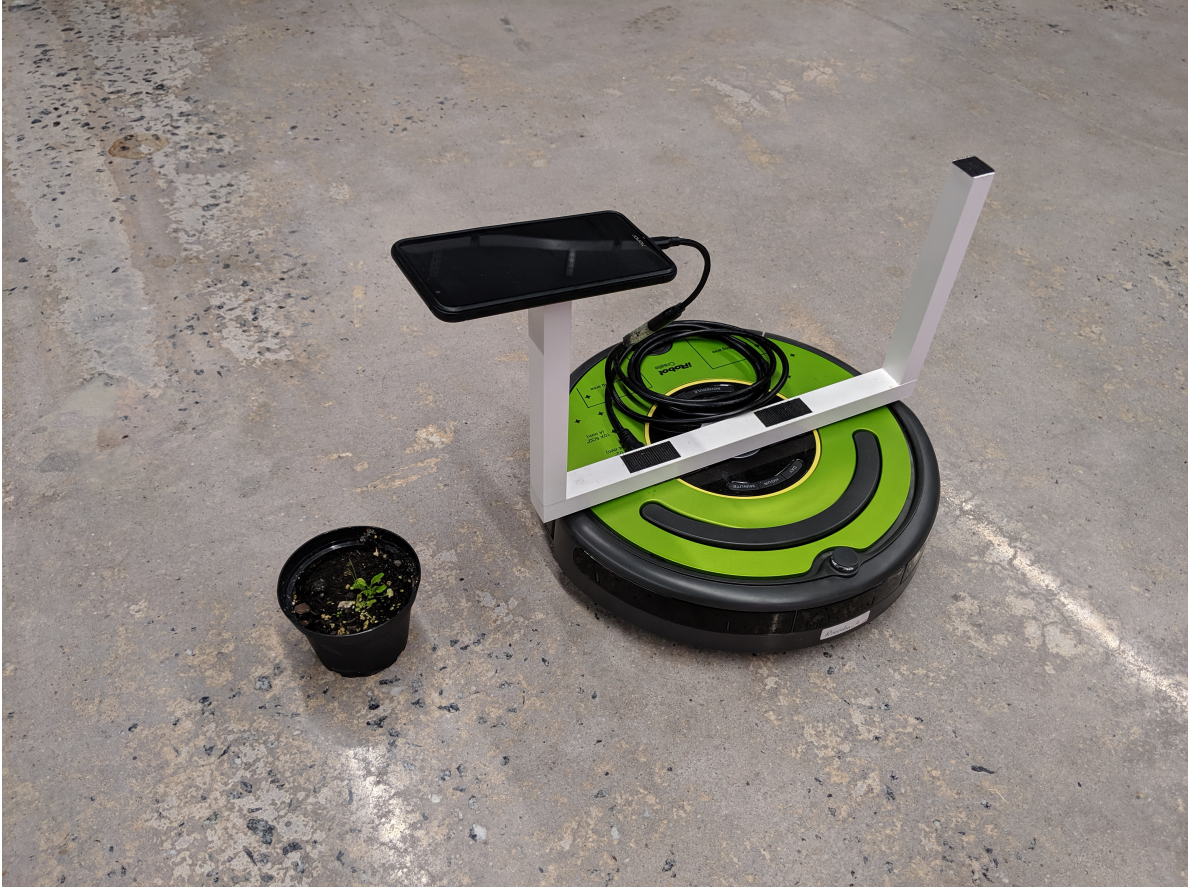
Figure 2.7: Robotic implementation of deployed tiny-YOLOv3 model on Android Honor 7x phone and iRobot2 for data acquisition and real-time data processing.
