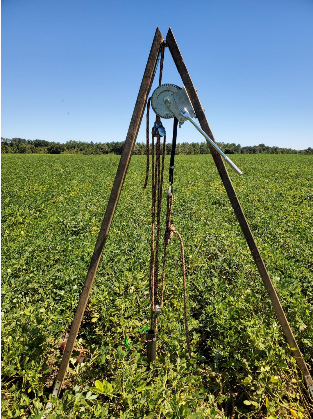
Fig. S1. Apparatus used to pull soil probe consisting of a hand winch, rope, and pulleys.
