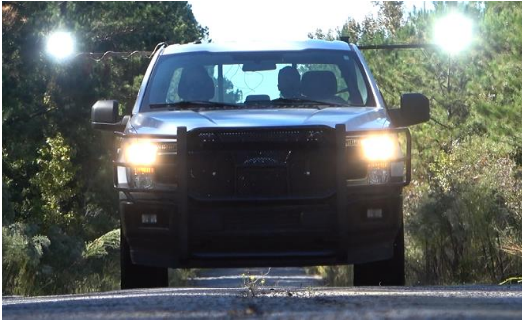
Figure 1. The experimental vehicle with airplane landing lights attached.
