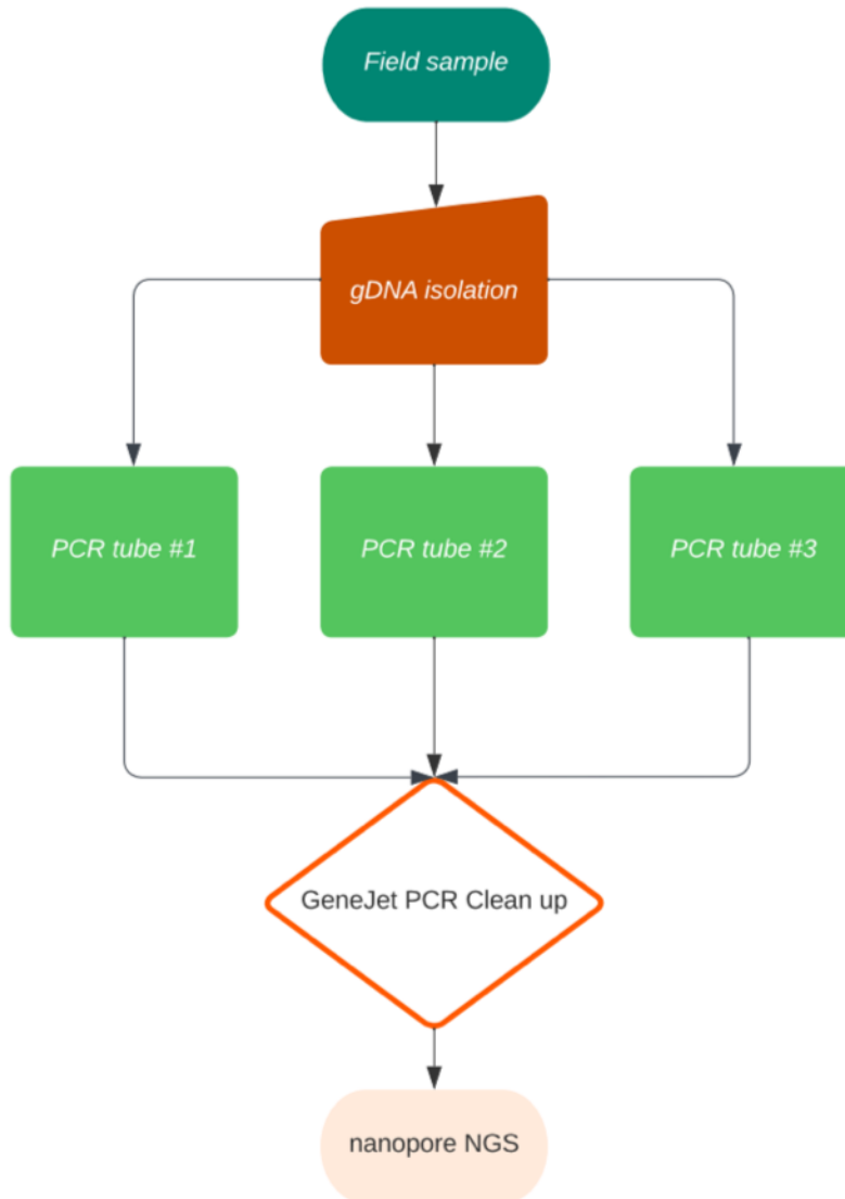
Figure 4-1. A simple workflow for 1 nanopore NGS run. This sequencing workflow was performed in triplicate for 18S, ITS1, and CO1 DNA regions.
