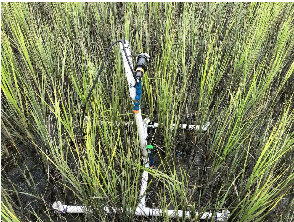
Figure 3.4 Field picture of leaf-level ChlF measurement system that installed on a custom-made PVC frame that supports ChlF measurements from S. alterniflora at the top and bottom of the plant canopy
