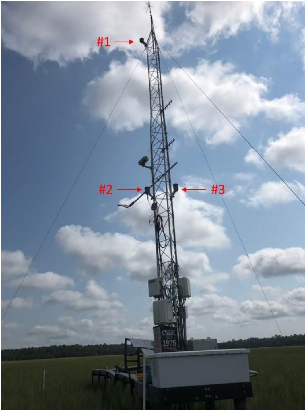
Figure 3.7 GCE-LTER flux tower with sensor positions marked with numbers. The positions of interest to our study are #1: air temperature sensor at the top of the tower (107 thermocouple);
