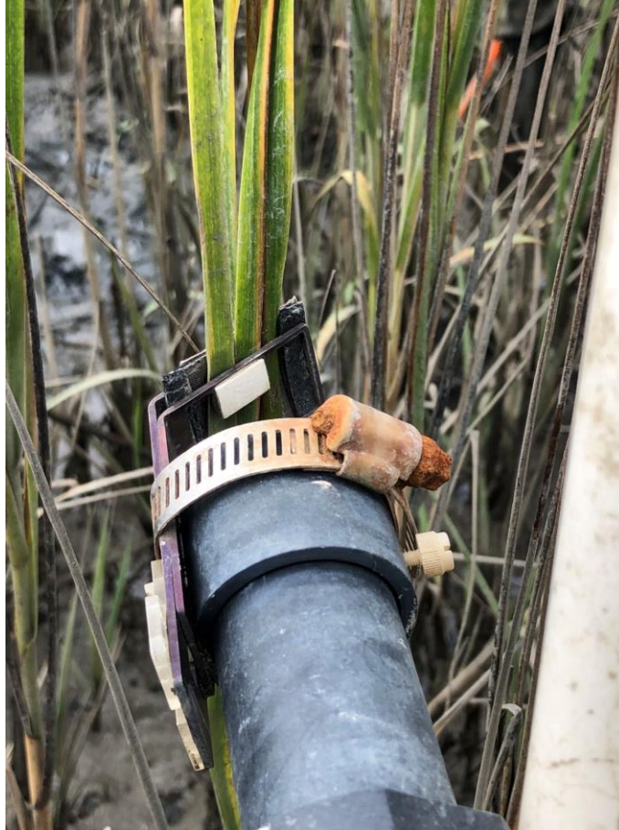
Figure 3.2 a detailed view of the MONI – HEAD measuring head in the field with three S. alterniflora leaves selected in the sampler clip.
