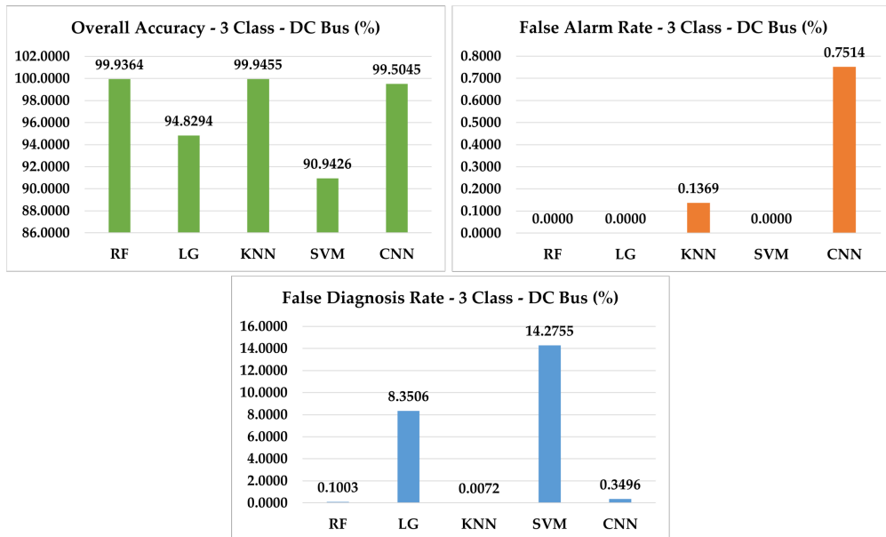
Figure 5.12: Overall accuracy, false alarm rate, and false diagnosis rate for 3-class DC bus system monitor.
