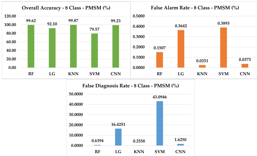
Figure 5.6: Overall accuracy, false alarm rate, and false diagnosis rate for 8-class PMSM individual monitor.
