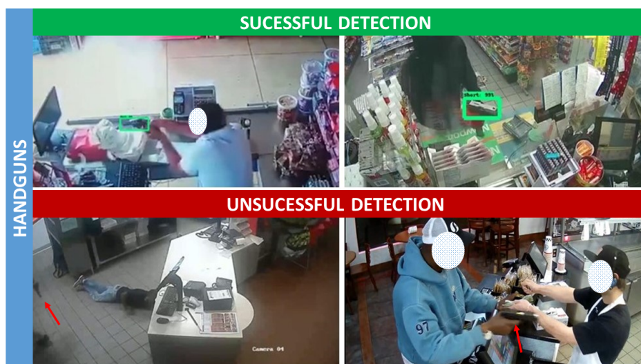
Figure 4.30: Examples of successful (top) and unsuccessful (bottom) detection of hand guns.
