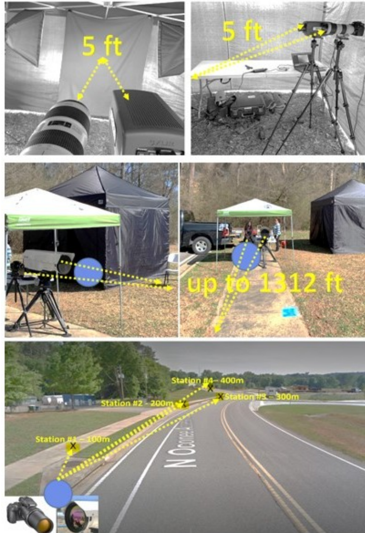
Figure 3.1: Overview of the data collection location and equipment setup.
