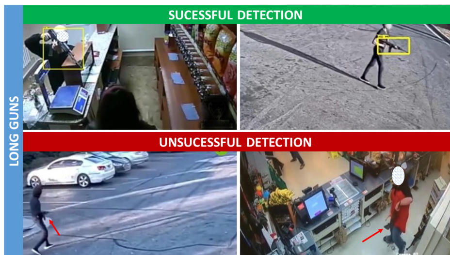
Figure 4.29: Examples of successful (top) and unsuccessful (bottom) detection of long guns.
