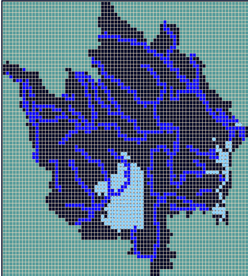
Figure 3.11: Numerical model with finite-difference grid and relevant boundary conditions.
