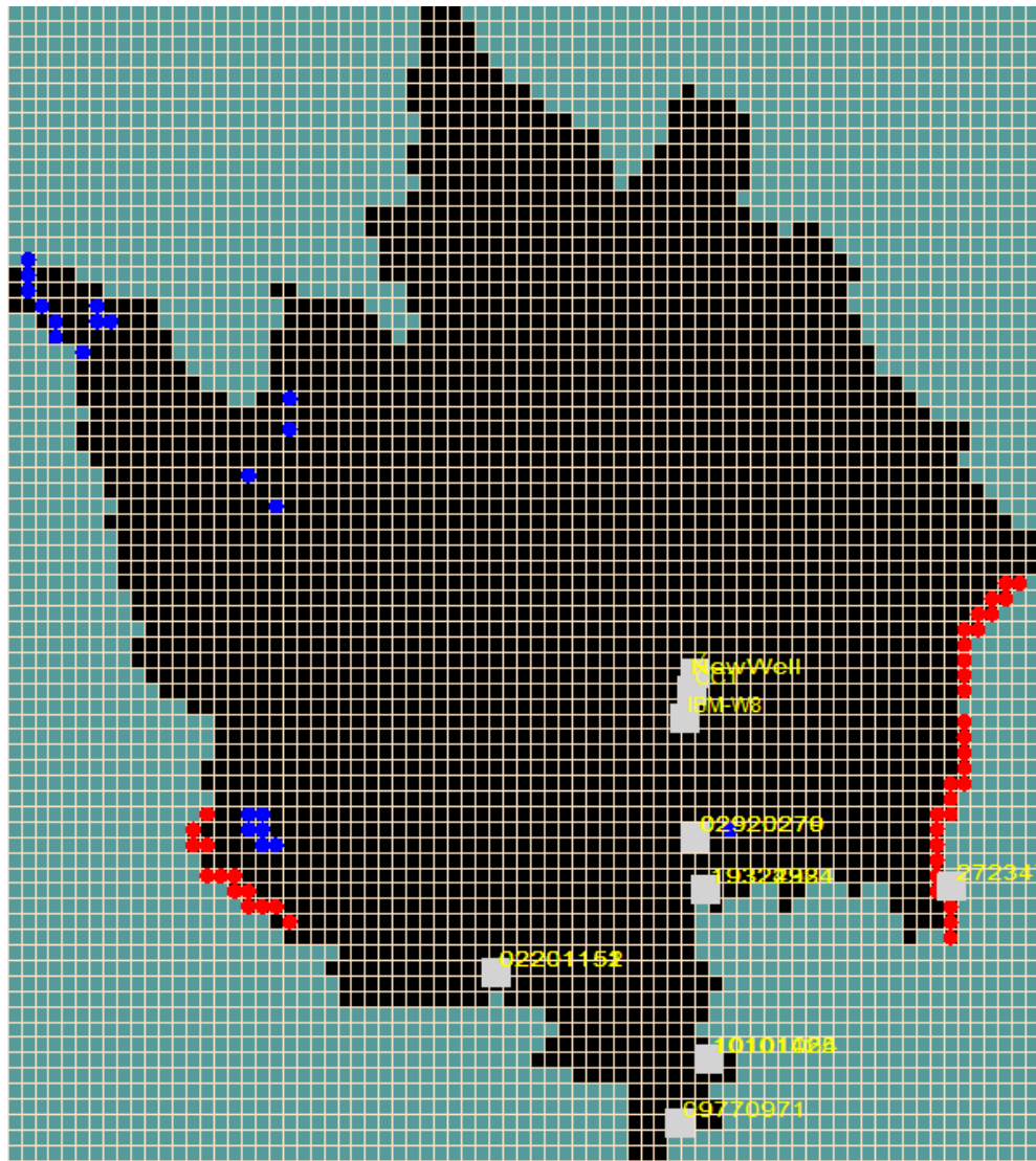
Figure 3.10: Constant head boundary conditions (red) in layer 2 of the regional steady-state model.
