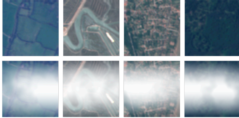
Figure 3.3: EuroSAT data points before (top row) and after (bottom row) adding cloud layers.
