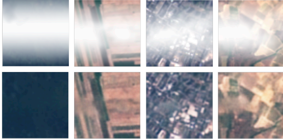
Figure 3.6: Output (bottom row) of the cloud removal module when it is fed with cloudy data (top row).
