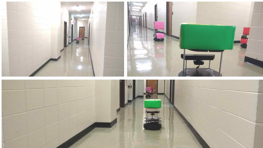
Figure 7.5: (top-left) Patrollers (in pink and red) in the longer hallway of instance 2 of the domain. (top-right) Learner’s (green) perspective as it observes the patrollers from its vantage point. (bottom) Learner penetrating the patrol to reach the goal undetected (first door on its right). The learner perceives the location and the orientation of each patroller by using the depth and the bounding box for color blob detected via CMVision.
