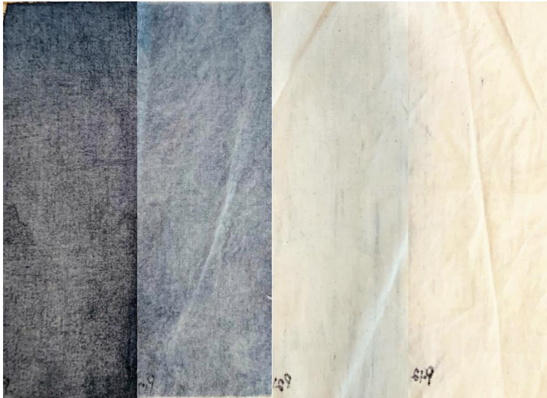
Figure 3.8: Optical images of coated samples 1% chitosan (wof)+6% NI dispersion (washed and unwashed), 1% (vow) chitosan+ 6% NI dispersion (washed and unwashed)
