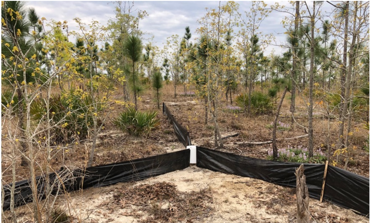
Figure 3.2. Modified AHDriFT system at Alapaha River Wildlife Management Area in Irwin County, Georgia, USA. The wildlife camera housing sits in the center of the Y-shaped drift fence array.
