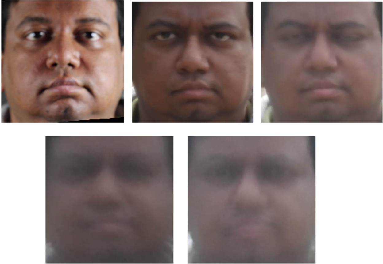
Figure 4.4: Geometrically normalized images. Top row - indoor, 100 and 200 meters. Bottom row - 300 and 400 meters.
