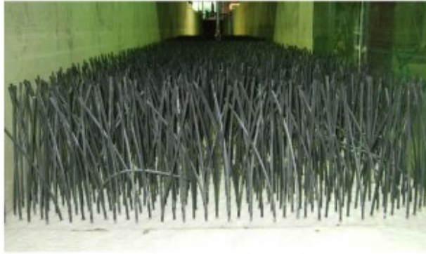
Figure 2.3: Artificial Spartina alterniflora array in a flume used to run simulations for real-life scenarios (Anderson & Smith, 2015).
