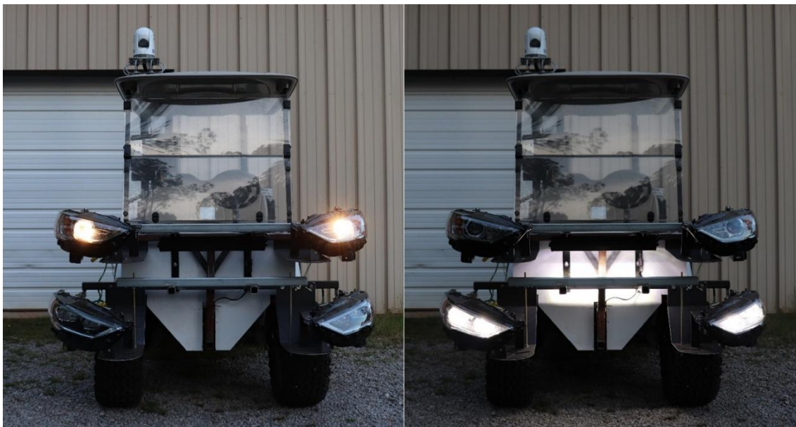
Figure 4.1. The electric golf cart used for our trials was outfitted with two sets of stock 2017-2020 Ford Fusion headlights (tungsten-halogen and light emitting diode), a rear-facing lightbar, and a forward-looking infrared camera for behavioral recording. Images display tungsten-halogen, low-beam, lightbar off (left) and light emitting diode, high-beam, lightbar on (right) treatments.
