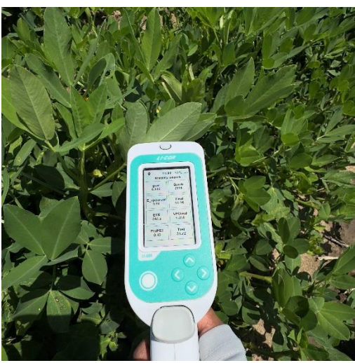
Figure 3.2. Measurement of physiological parameters of peanut using LI-600 porometer/fluorometer.
