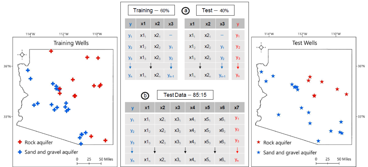
Figure 6. Model design showing train/test split ratios for the spatial (a) and temporal (b) evaluations and the locations of the split wells.
